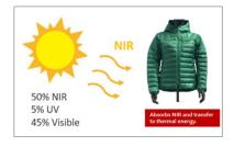
3. FUN-MAX<sup>®</sup>HL Light Heat Series: This series utilizes metal oxides to absorb sunlight or near-infrared rays emitted by the human body, converting them into heat energy, providing a warm sensation.
